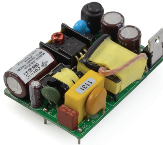
FIGURE 5: The CUI medical power supply family (15~400 W) is certified for IEC 60601-1 2 nd edition and 3 rd edition two MOPP standards.
