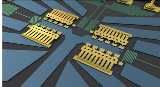
Figure 4. Close-up graphic showing four MEMS cantilever switch beams (SP4T configuration).
