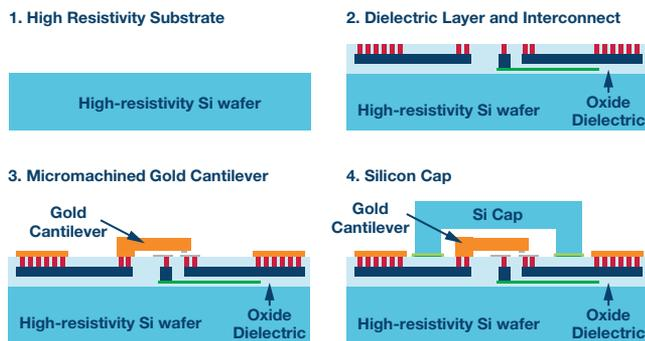
Figure 3. MEMS switch fabrication overview.
