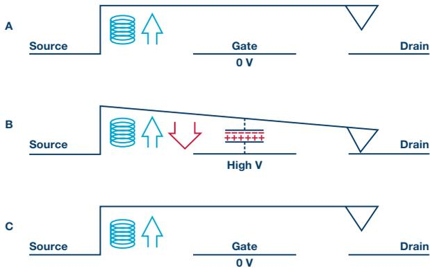
Figure 2. MEMS switch actuation process, A and C show the switch turned off, B shows it turned on.
