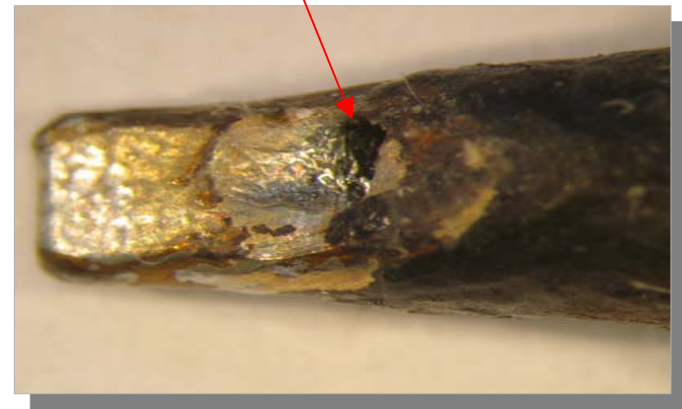
LTC Soldering Tip “Eroded”
