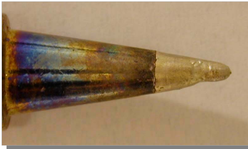
Soldering tip after 10,000 cycles with Lead Free SAC
