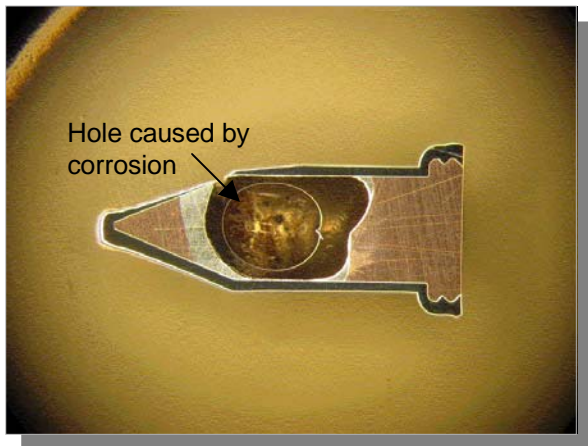
Cross section of a degraded LTC soldering tip
