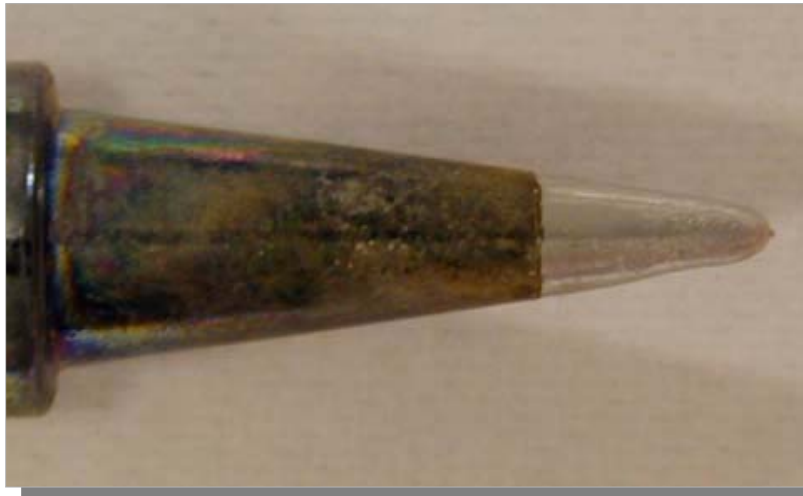
Soldering tip after 20,000 cycles with Sn / Pb
